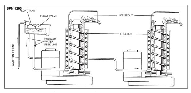
By running the ice maker, i.e. by putting the unit under power, starts the automatic and continuous icemaking process which would not stop until the ice storage bin gets filled-up to the level of the control "eyes" located on the ice chute. As the ice level raises to interrupt the light beam running between the two infrared leds (one or both on model SPN1205), the unit stops after six seconds, with the simulteneous glowing of the YELLOW LED signalling the "Full Bin" situation.
