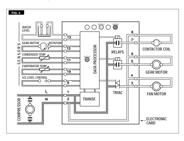
This will cause a gradual decrease of the water level in the float reservoir and as soon as the level gets below the two vertical metal pins, the flaker stops to operate and the **YELLOW warning LED** will glow to signal the shortage of water (Fig. 4)
