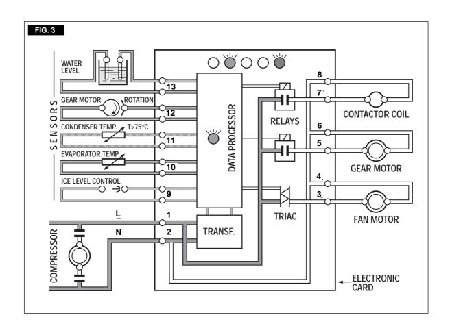
**NOTE**. If, after ten minutes from the compressor start-up, the evaporating temperature has not dropped down to a value lower than -1°C (30°F) the evaporating temperature sensor detects such an abnormal situation and stops consequently the unit operation.
