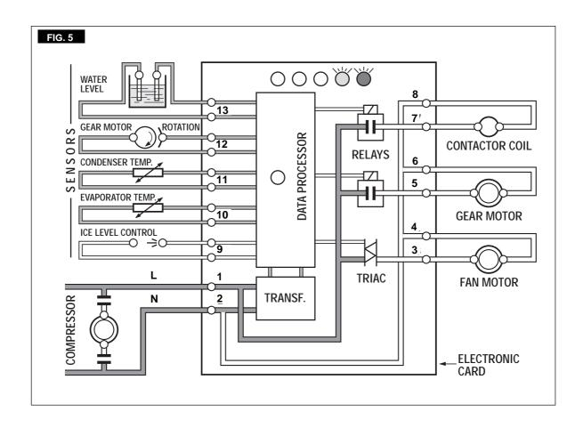
NOTE. The ICE LEVEL CONTROL (INFRARED SYSTEM) is independent of the temperature however, the reliability of its detection can be affected by external light radiations or by any sort of dirt and scale sediment which may deposit directly on the light source and on the receiver.
